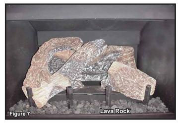
**Log #4 (SRV2113-703)**: Locate the notch on the bottom of log # 4. Mate the notch with the shoulder screw that is located on the burner top. Mate the rear groove with the far right grate tine as shown above. Apply the supplied lava rock as shown above.
